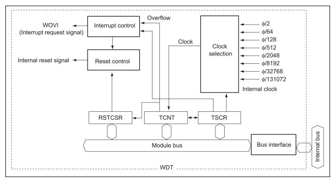
Figure 1 Block Diagram of Interval Timer
