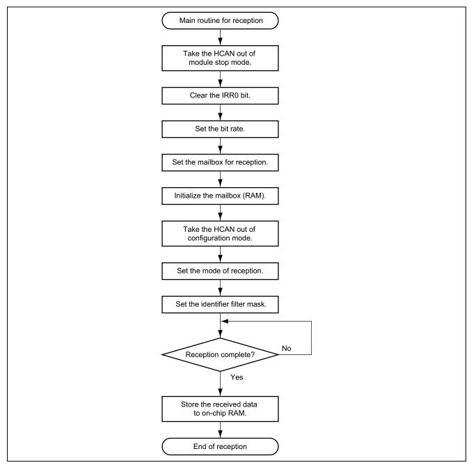
Figure 2 Flowchart for the Receiver
