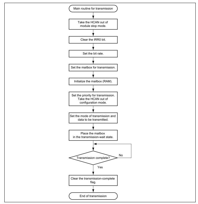
Figure 1 Flowchart for the Transmitter
