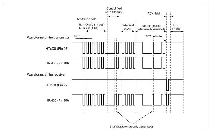
Figure 3 Waveforms during Operation
