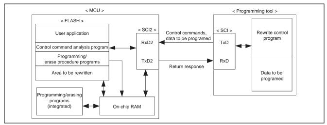
Figure 1 Block Diagram of On-Board Reprogramming Setup using an SCI (asynchronous mode)
