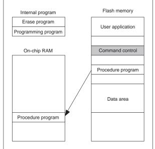
(4) While running on the on-chip RAM, the procedure program downloads a built-in program (programming program) onto the onchip RAM to temporarily store the write data being received from the programming tool, and then programs this latter into the flash memory starting from the specified start address in 128-byte blocks.
