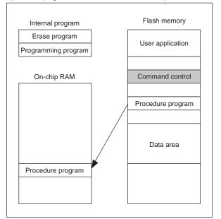
(3) The procedure program running on the on-chip RAM downloads a internal program (erasing program) into the on-chip RAM. The downloaded program erases the flash memory in the specified block area.
