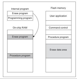
(4) The procedure program running on the on-chip RAM then downloads the built in program (programming program) into the on-chip RAM, outputs a write data request signal to the programming tool, stores the write data received from the programming tool into the on-chip RAM once, and then programs the data in 128-byte blocks, beginning with the specified start address on the flash memory.
