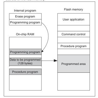
Figure 3 Explanation of Software Operation
