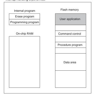
(2) In IRQ0 interrupt handling, the flash erase/programming procedure program is transferred to the on-chip RAM, and the procedure program is executed on the same on-chip RAM.
