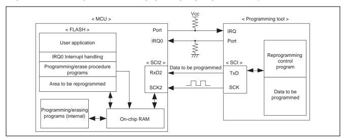
Figure 1 Block diagram of on-board reprogramming setup using an SCI (clock synchronous mode)
