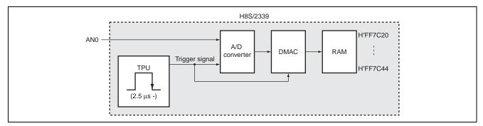
Figure 1 Block Diagram of A/D Conversion by Timer Trigger
