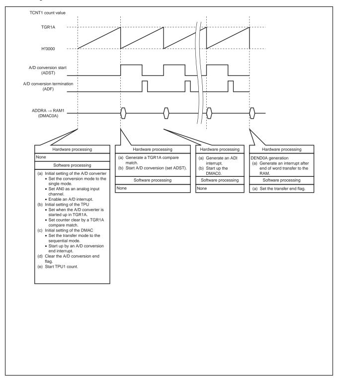
Figure 3 Principles of Operations Used of A/D Conversion by Timer Trigger
