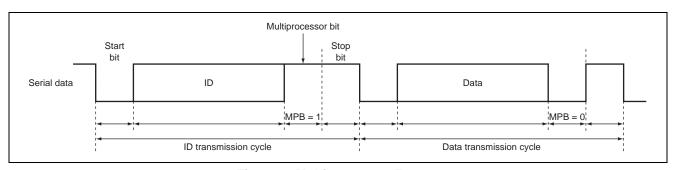
Figure 2 Multiprocessor Format
