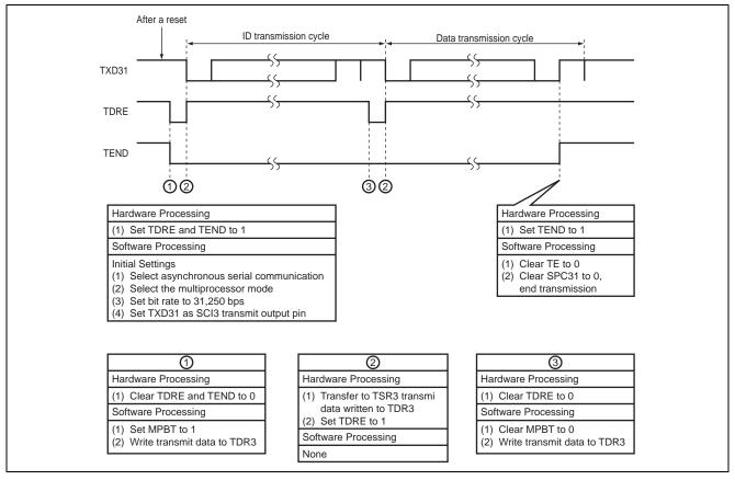
Figure 4 Principles of Operation for Multiprocessor Serial Data Communication
