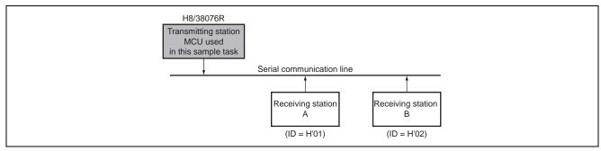
Figure 1 Communication Between Processors Using Data Transfer in Multiprocessor Format
