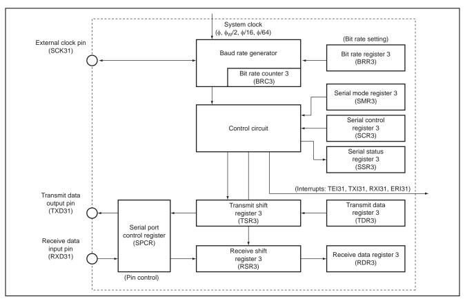
Figure 3 Block Diagram of SCI3
