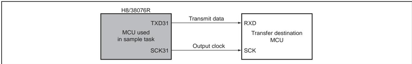
**Figure 1 Serial Data Transmission (Master Transmission) in the Clock-Synchronous Mode**
