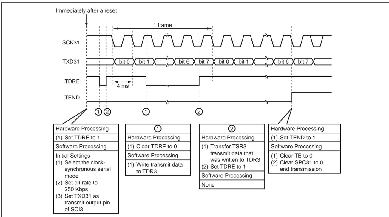
Figure 3 Principles of Operation for Serial Data Transmission in the Clock-Synchronous Mode
