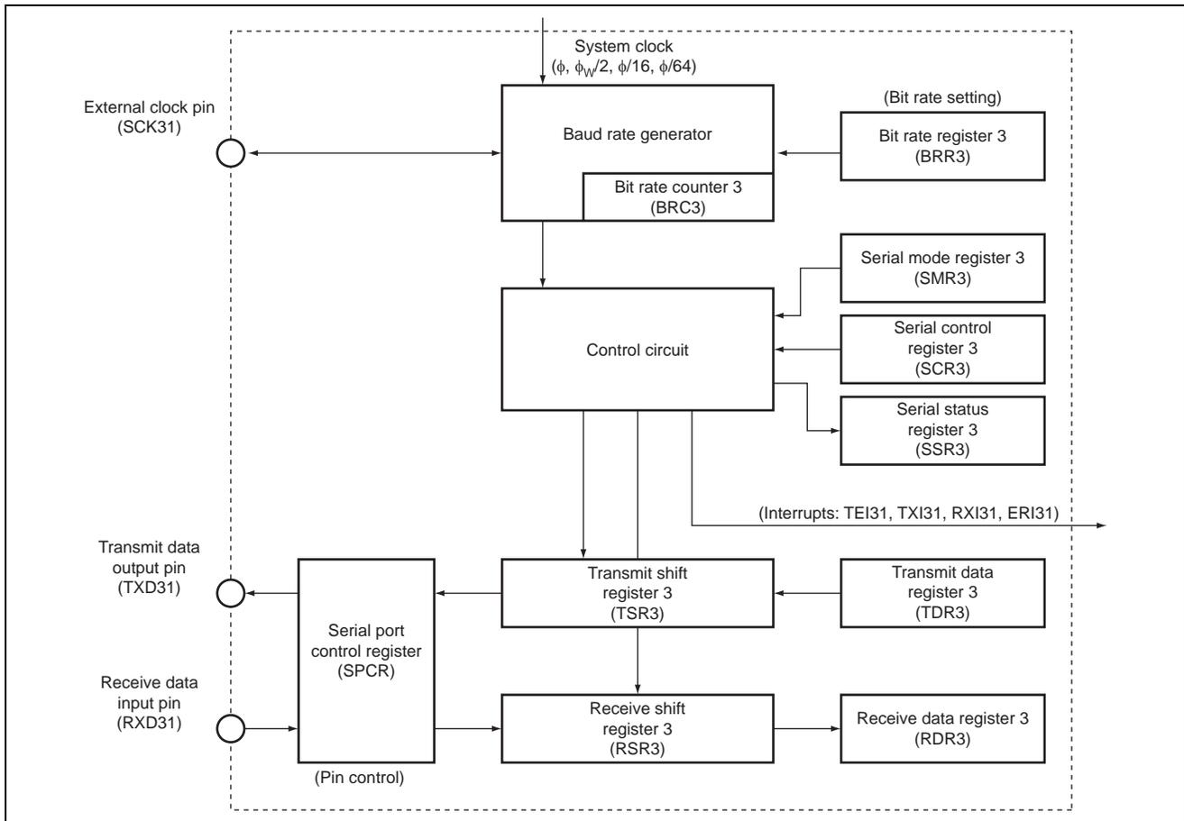
**Figure 2 Block Diagram of SCI3**
