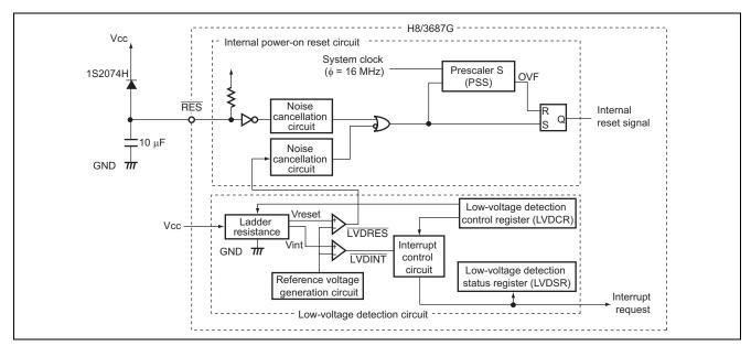
Figure 2.1 Block diagram of the low-voltage detection circuit
