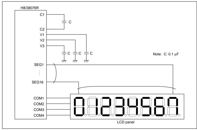
Figure 1 Example of LCD Panel Connection
