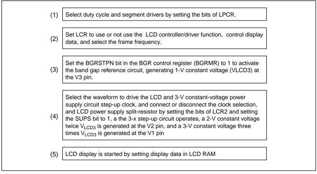
Figure 4 Setting Procedure when Using 3-V Constant-Voltage Power Supply Circuit
