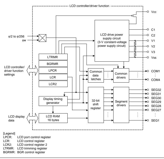
Figure 2 Block Diagram of LCD Controller/Driver
