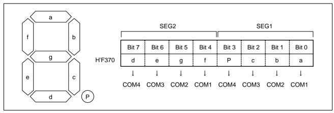
Figure 8 Relationship of LCD RAM Set Values and LCD Display/Non-Display
