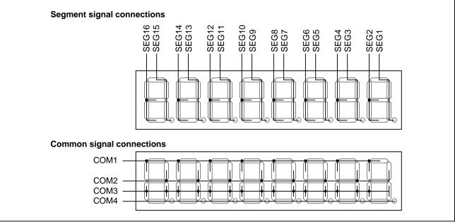
Figure 5 LCD Panel Segment Signal and Common Signal Connections
