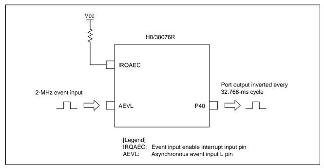
Figure 1 Example of Event Counter Operation in the 16-Bit Mode
