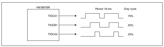
Figure 1 Example of 3-Phase PWM Output Using PWM Mode 2 Function
