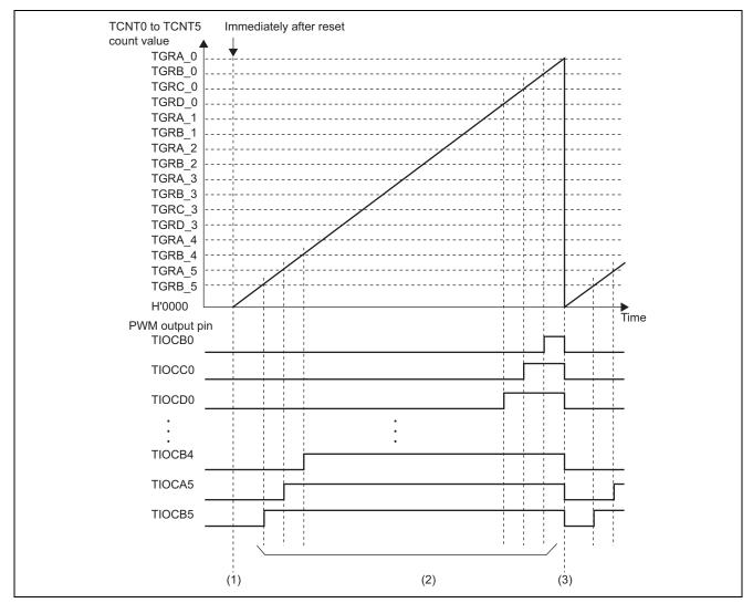
Figure 3 Operation of 15-Phase PWM Output
