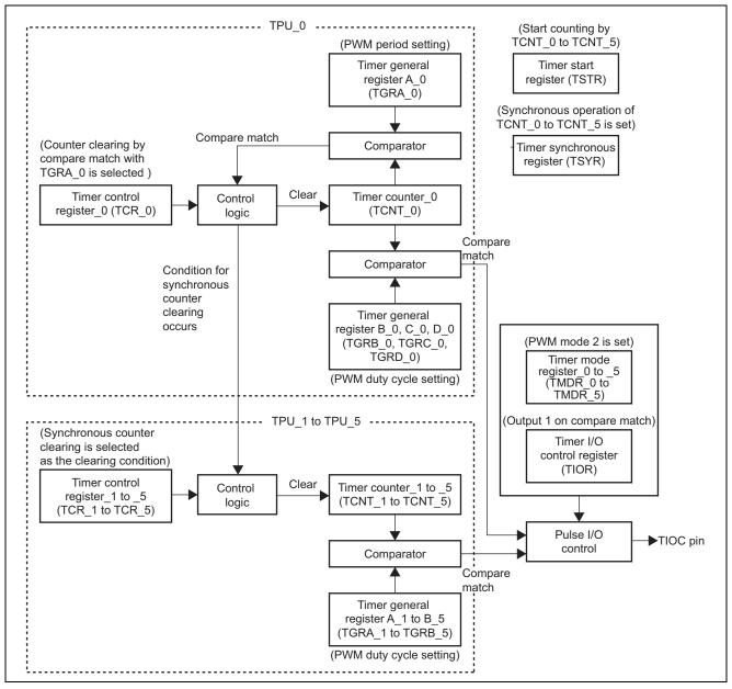
Figure 2 Block Diagram of 15-Phase PWM Output
