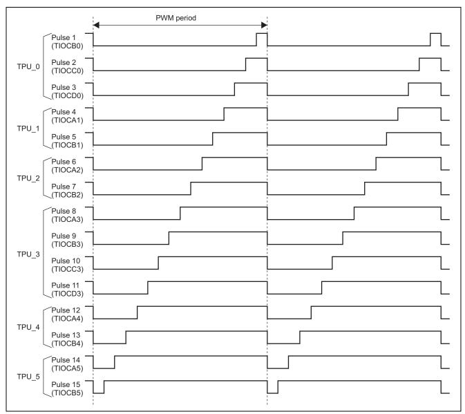
Figure 1 Example of 15-Phase PWM Output
