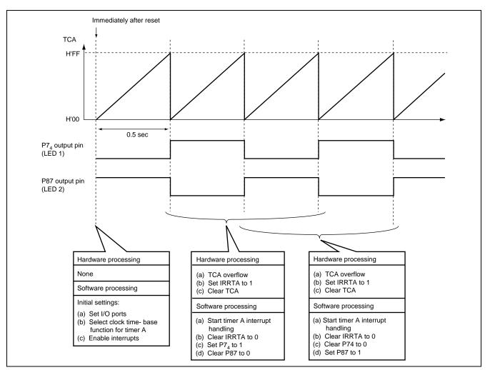
Figure 3.1 Operation Principle: Making LEDs Connected to I/O Ports Flicker
