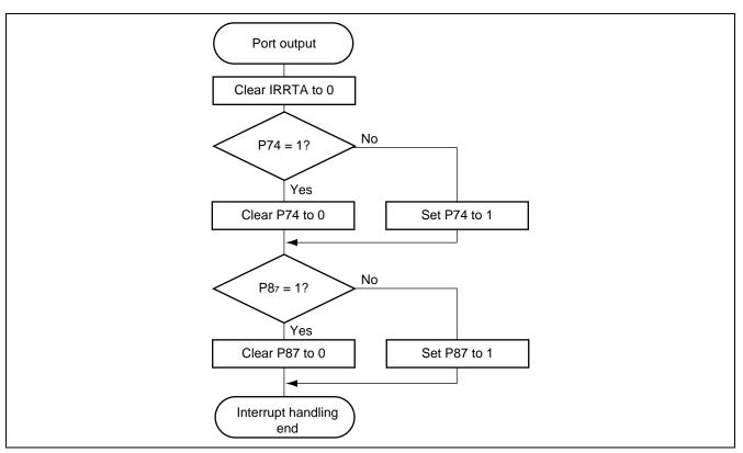
Figure 5.2 Flowchart for Timer A Interrupt Handling Routine
