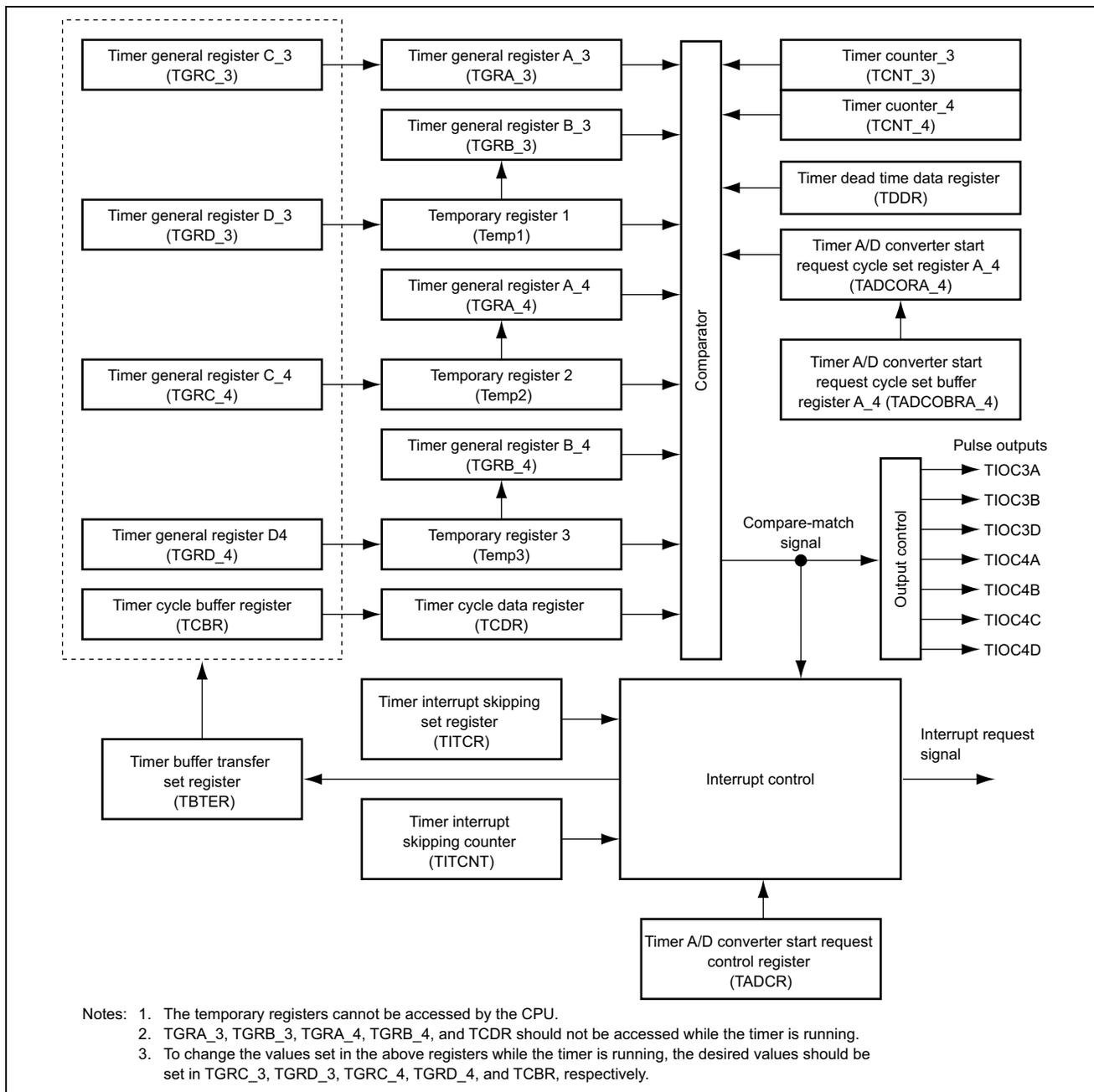
**Figure 3 Block Diagram of Channels 3 and 4 of MTU2 when External Pulse Width Measurement Feature of Channel 5 is Used**
