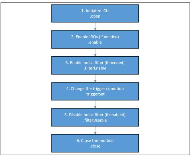
Figure 3 Typical External IRQ HAL Module Application Flow Chart
