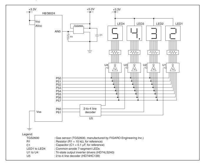
Figure 1 Hardware Configuration
