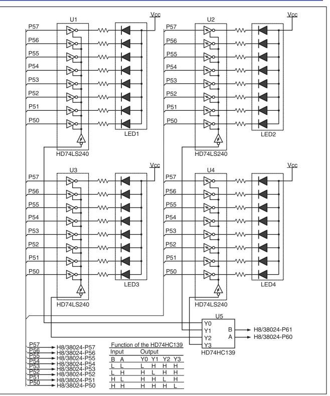
Figure 4 Method of Controlling 7-Segment LEDs
