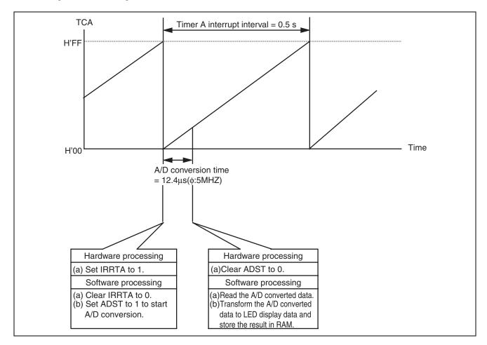
Figure 8 Description of A/D Conversion of the AN0 Pin Signal when Timer A is Used
