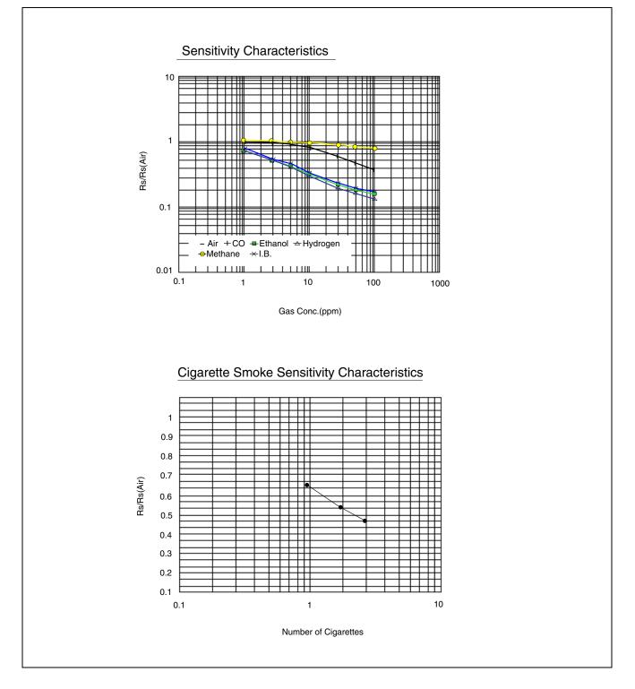
Figure 3 Sensor Sensitivity Characteristics (Reference Values)
