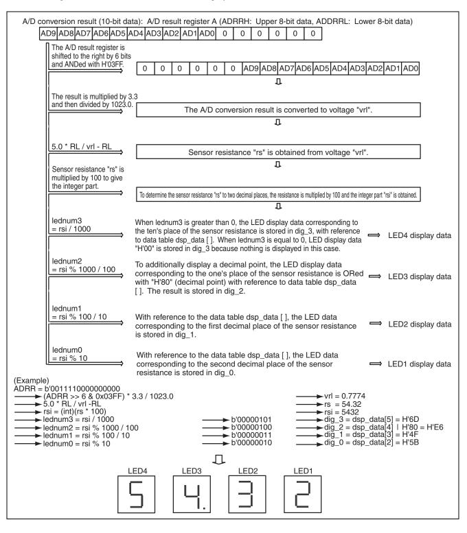
Figure 5 How the Resistance is Displayed on the LEDs
