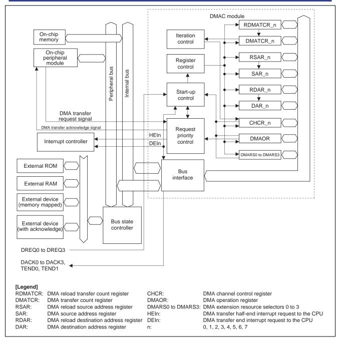
Figure 2 Block Diagram of the DMAC
