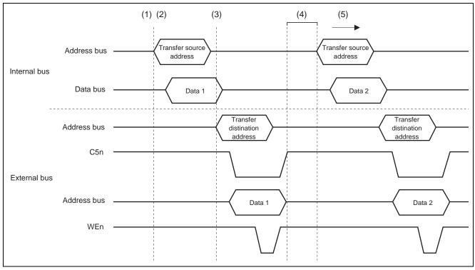
Figure 4 Operation in Dual Address Mode
