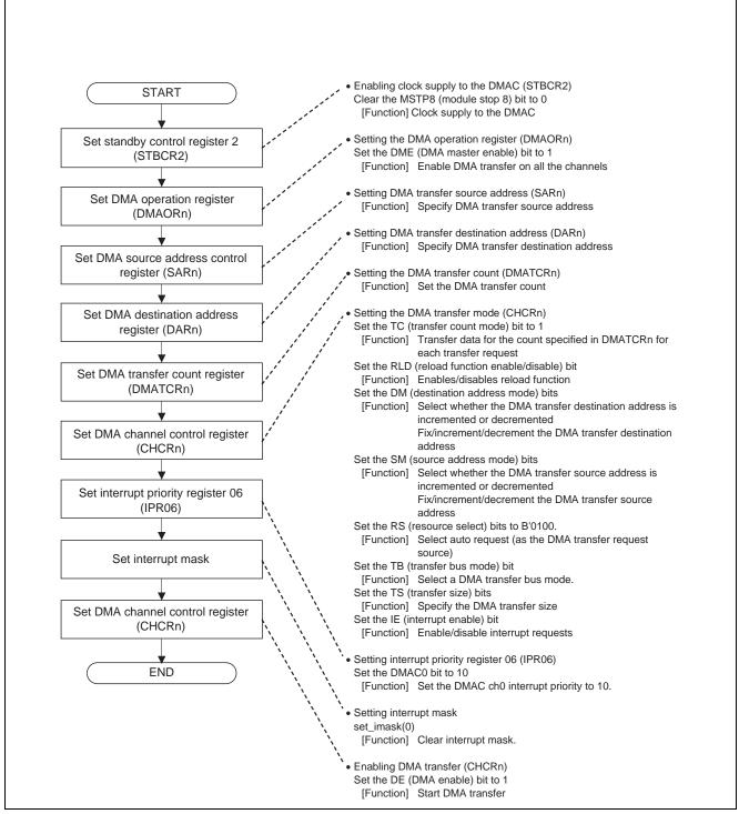
Figure 3 Flowchart of Initializing DMAC
