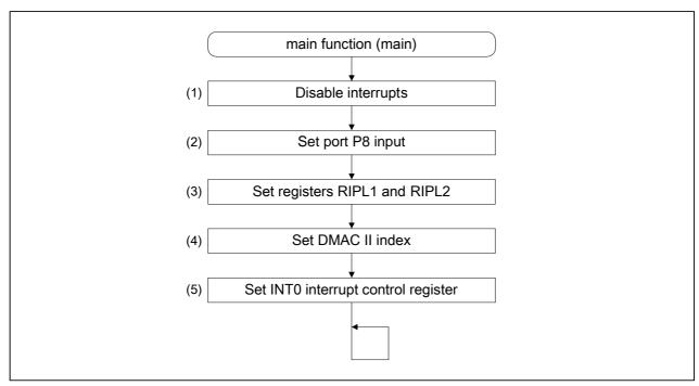
Figure 5.1 Main Function Flowchart
