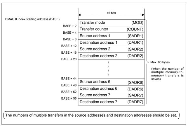
Figure 4.1 Configuration of the DMAC II Index
