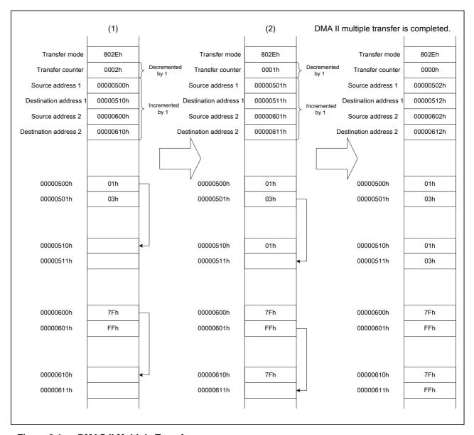
Figure 3.1 DMAC II Multiple Transfer
