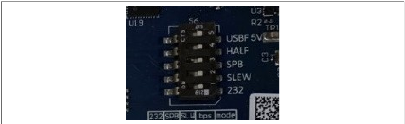
Figure 9 The setting of DIPSW S6 for the DK-S3A7
