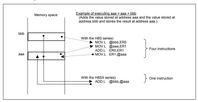
Figure 1 Example of Adding Data in Memory
