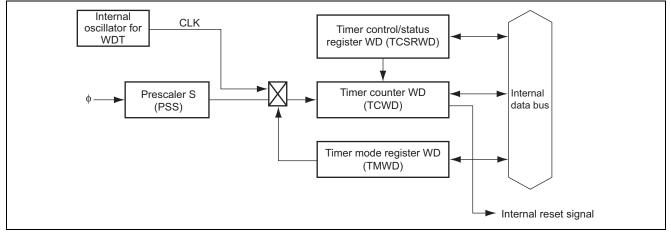
Figure 3 Block Diagram of the Watchdog Timer
