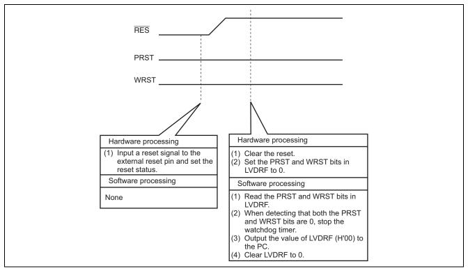
Figure 7 Operation of a Reset by the External Reset Pin RES
