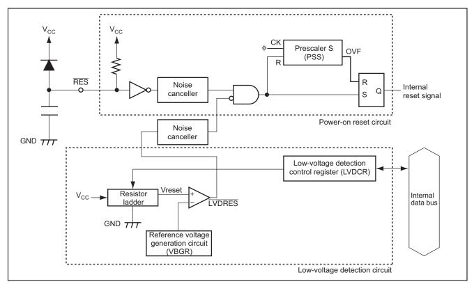
Figure 2 Block Diagrams of the Power-On Reset Circuit and the Low-Voltage Detection Circuit
