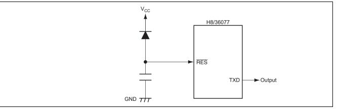
Figure 1 Connection Diagram of the H8/36077
