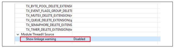
Figure 10 Disabling the Linkage Warning Error
