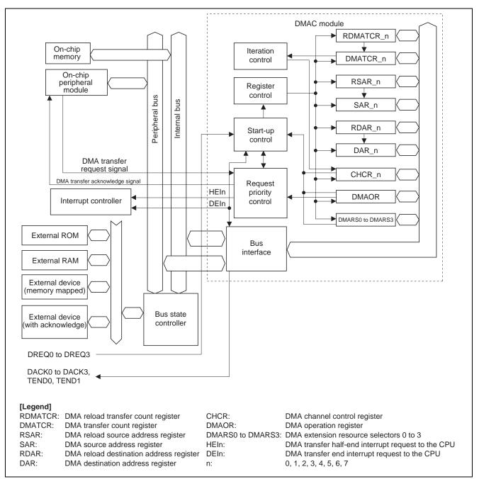
Figure 1 Block Diagram of DMAC
