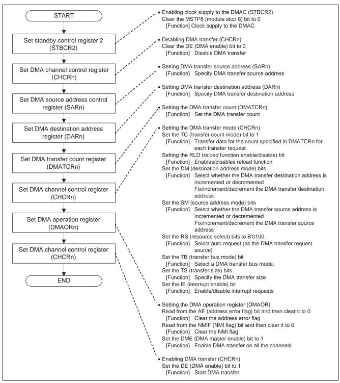
Figure 2 Flowchart of Initializing DMAC
