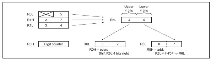
Figure 3 Dividing One Byte of Data in a General-Purpose Register into Two
