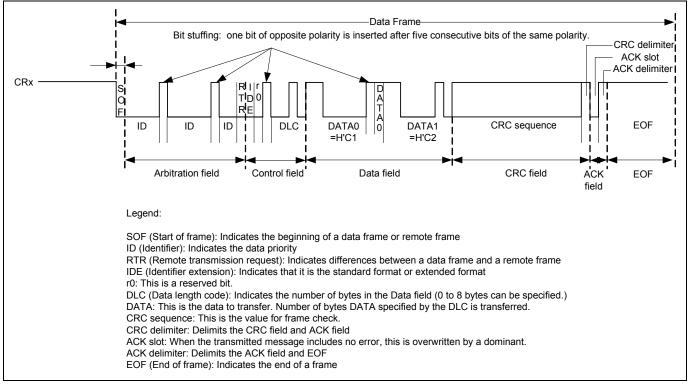
Figure 5 CAN Reception Waveform
