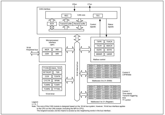
Figure 1 CAN Block Diagram (For One Channel)
