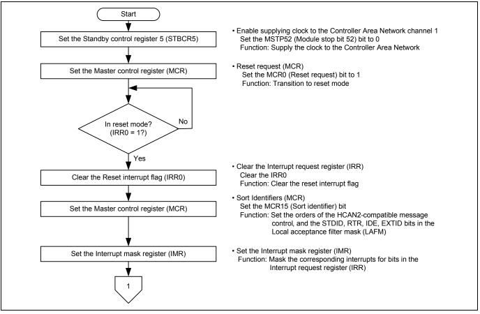
Figure 2 Flow Chart for Configuring the CAN Module (1/2)
