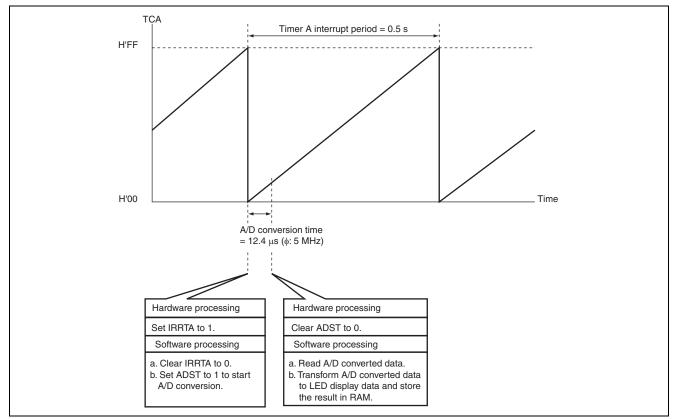
Figure 3.1 Operation Principle of A/D Conversion of AN0-Pin Signal Using Timer A
