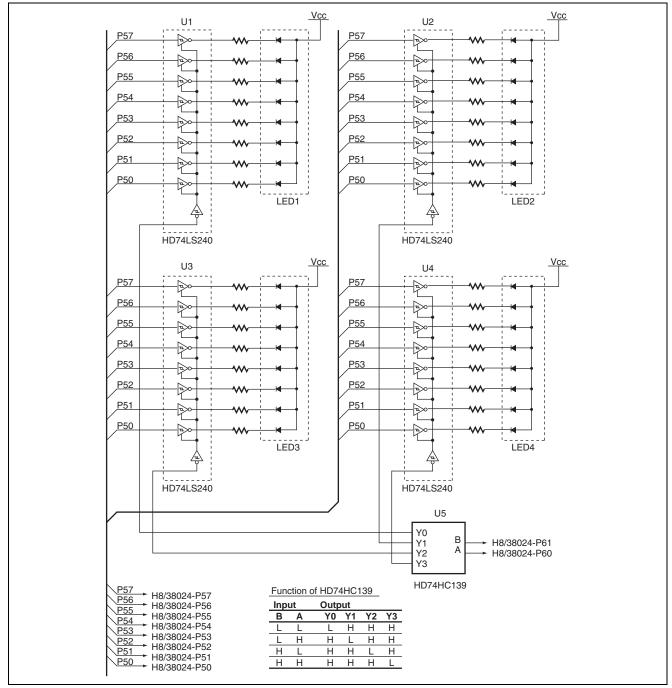
Figure 1.4 Control of 7-Segment LEDs
