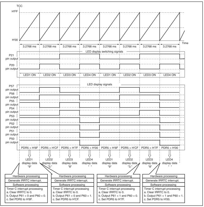
Figure 3.2 Operation Principle of 7-Segment LED Display Control
