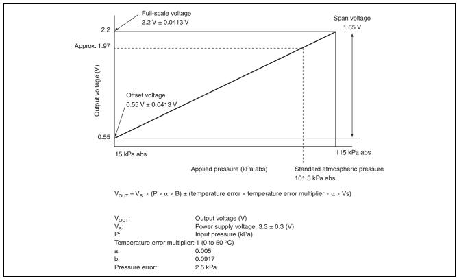
Figure 1.3 Output Characteristics (Reference)
