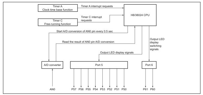
Figure 2.1 Block Diagram of Functions Used
