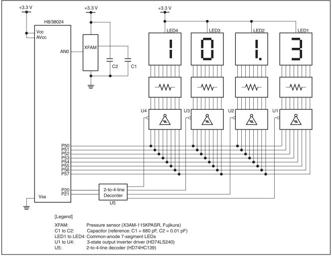
Figure 1.1 Hardware Configuration
