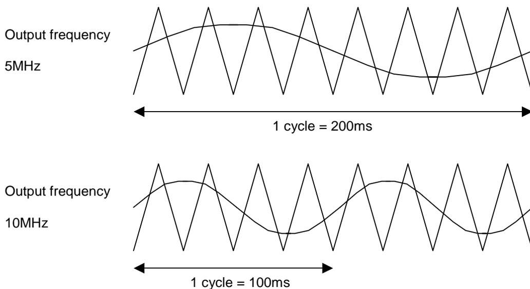
Figure 5.10 Altering the Output Frequency
