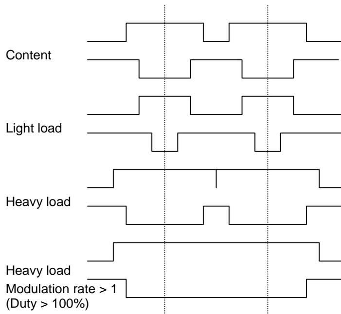
Figure 5.4 Relationship between Modulation Rate and Output Waveform
