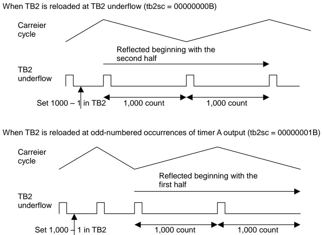
Figure 4.10 Carrier Cycle Settings and Refection
