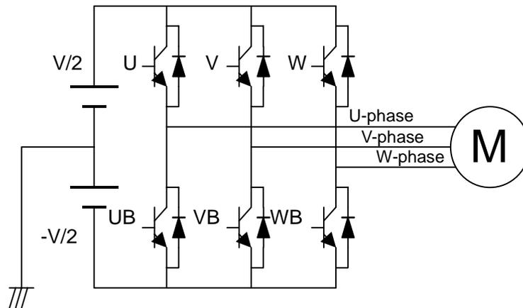
Figure 3.3 Power Transistor Circuit
