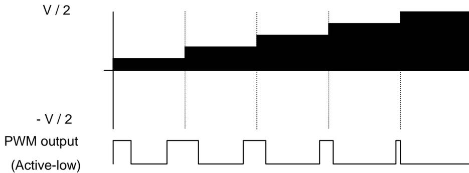
Figure 3.5 Changing an a.c. sine wave to a square wave by dividing it in time
