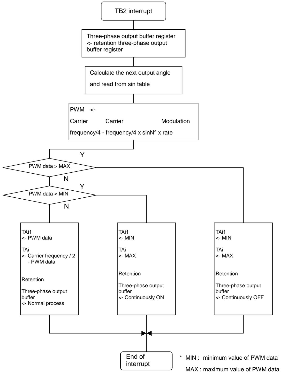
Figure 5.7 Example of a TB2 Interrupt Processing Flowchart (Method 1)
