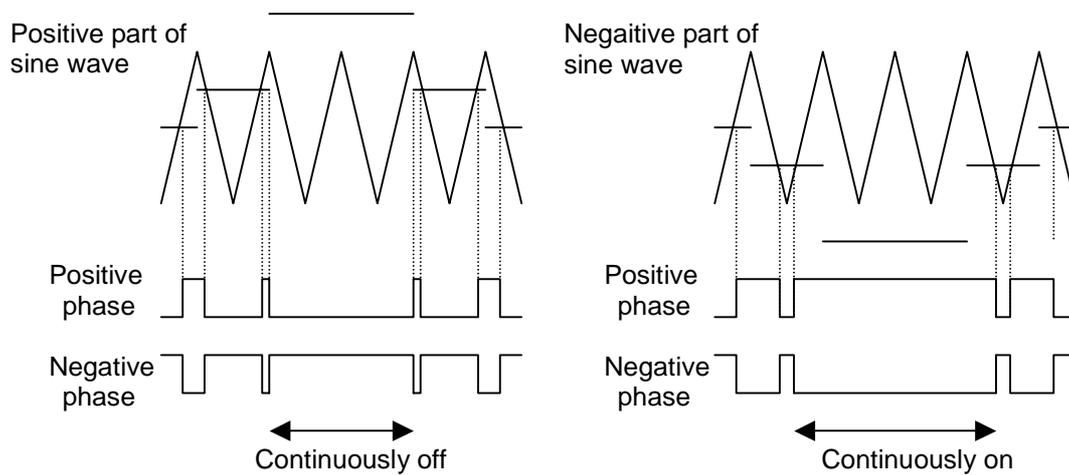
Figure 5.5 Conceptual Waveform of Two-phase Modulation Output
