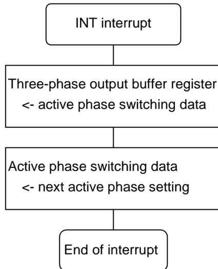
Figure 6.2 Sensor Interrupt and Output Phases
