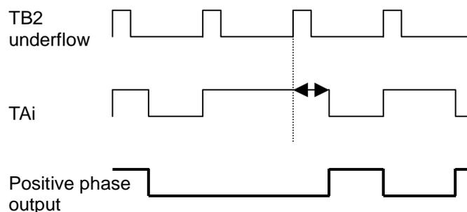
Figure 4.8 Output Waveform when TAI > TB2
