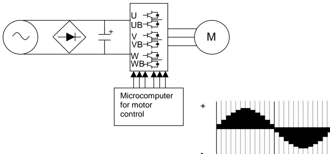
Figure 3.2 Example of Inverter Control Using a Microcomputer
