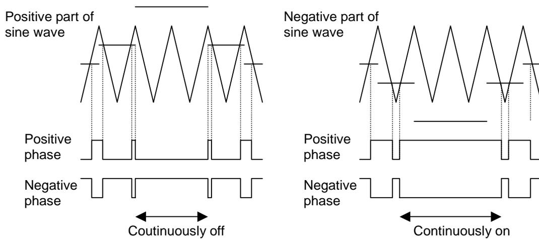
Figure 4.11 Conceptual Waveform of Two-phase Modulation Output (see Section 5 for details)
