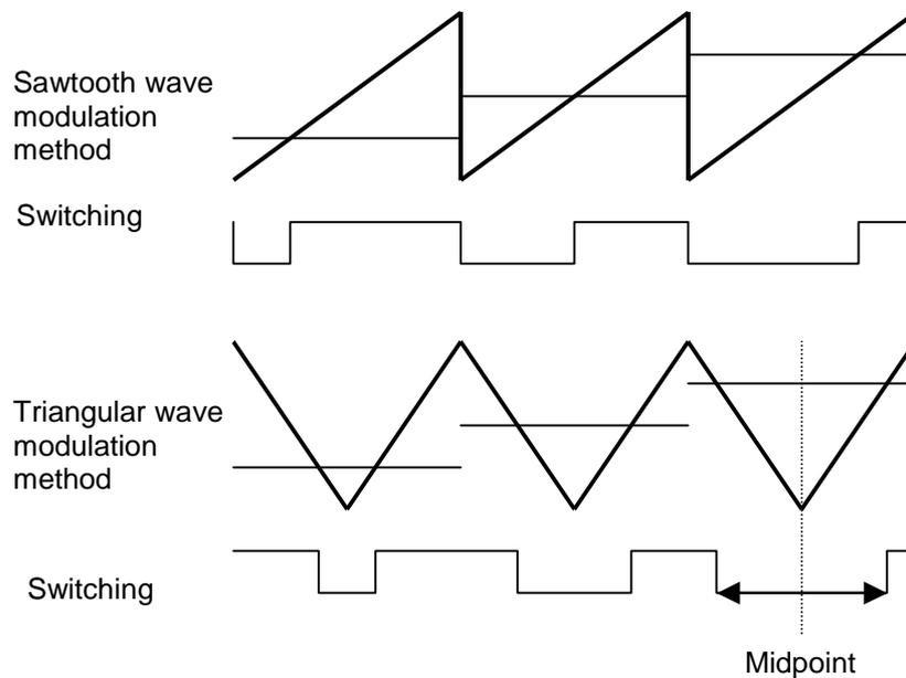
Figure 4.1 Carrier Frequency Modulation Method
