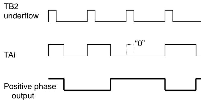
Figure 4.7 Positive Phase Waveform when TAI = 0
