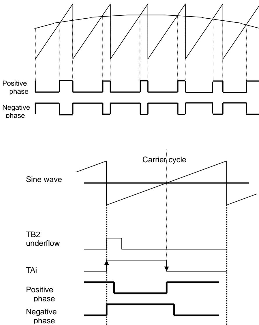
Figure 4.2 Relationship between Timer and PWM during Sawtooth Wave Modulation
