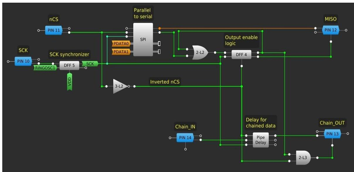
**Figure 7: SPI Interface and Data Chain Logic**
