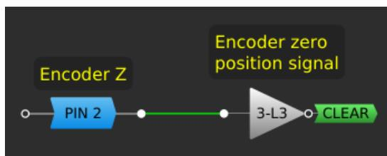
Figure 4: Logic for Z Input Signal
