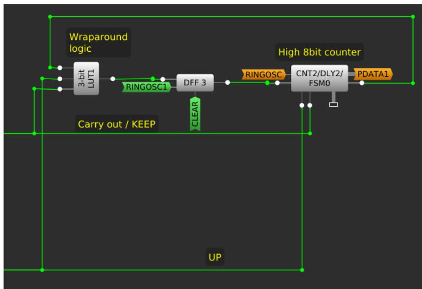
Figure 6: Wraparound Logic for High 8-bit Counter
