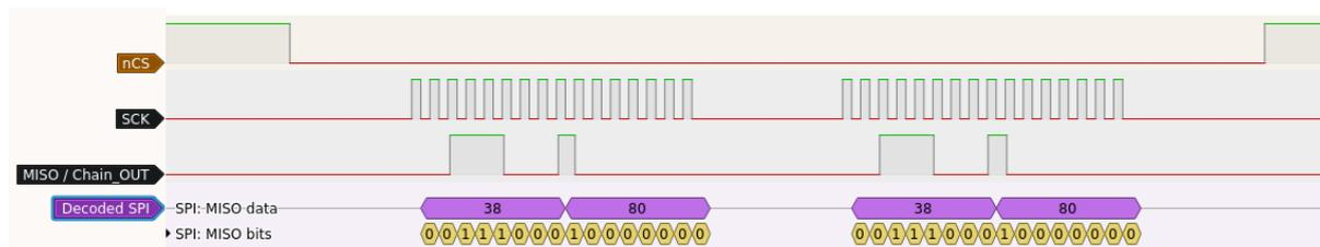
**Figure 8: SPI Signal Capture with Two Devices**
