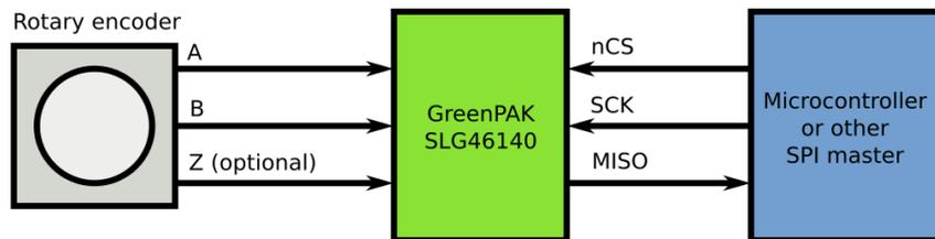
Figure 1: System Connections with One Encoder Device
