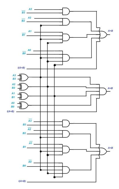
Figure 5: Magnitude Comparator Logic Diagram
