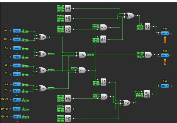
Figure 6: Magnitude Comparator Design
