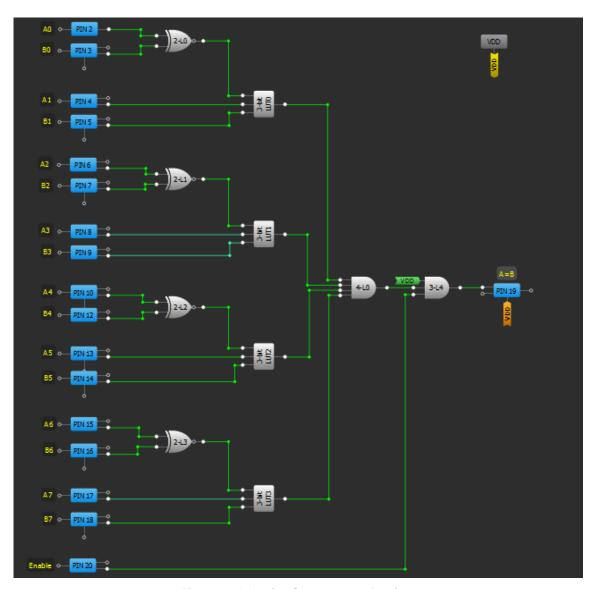
Figure 4: Identity Comparator Design
