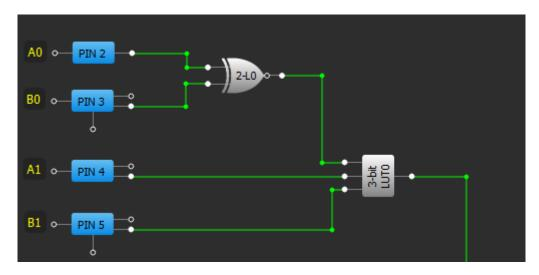
Figure 2: 2-Bit Identity Comparator Blocks
