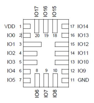
Figure 7: SLG46533V PINs Schematic
