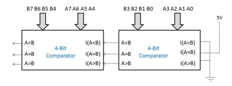
Figure 8: 8-Bit Magnitude Comparator Composition
