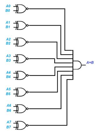
Figure 1: Logic Diagram of 8-Bit Identity Comparator
