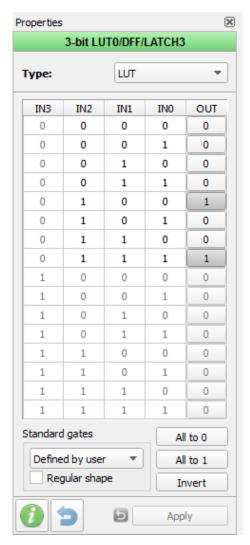
Figure 3: 3-bit LUT0 Configuration
