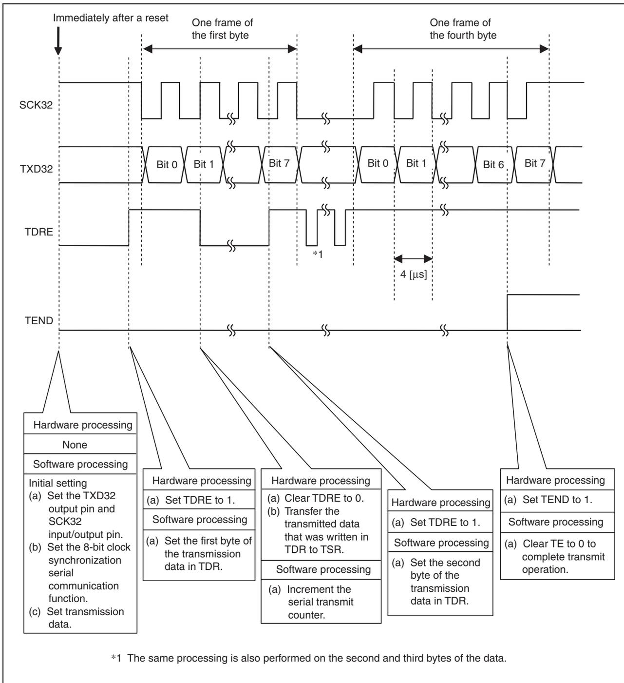
Figure 3 Operation during Transmission of Data
