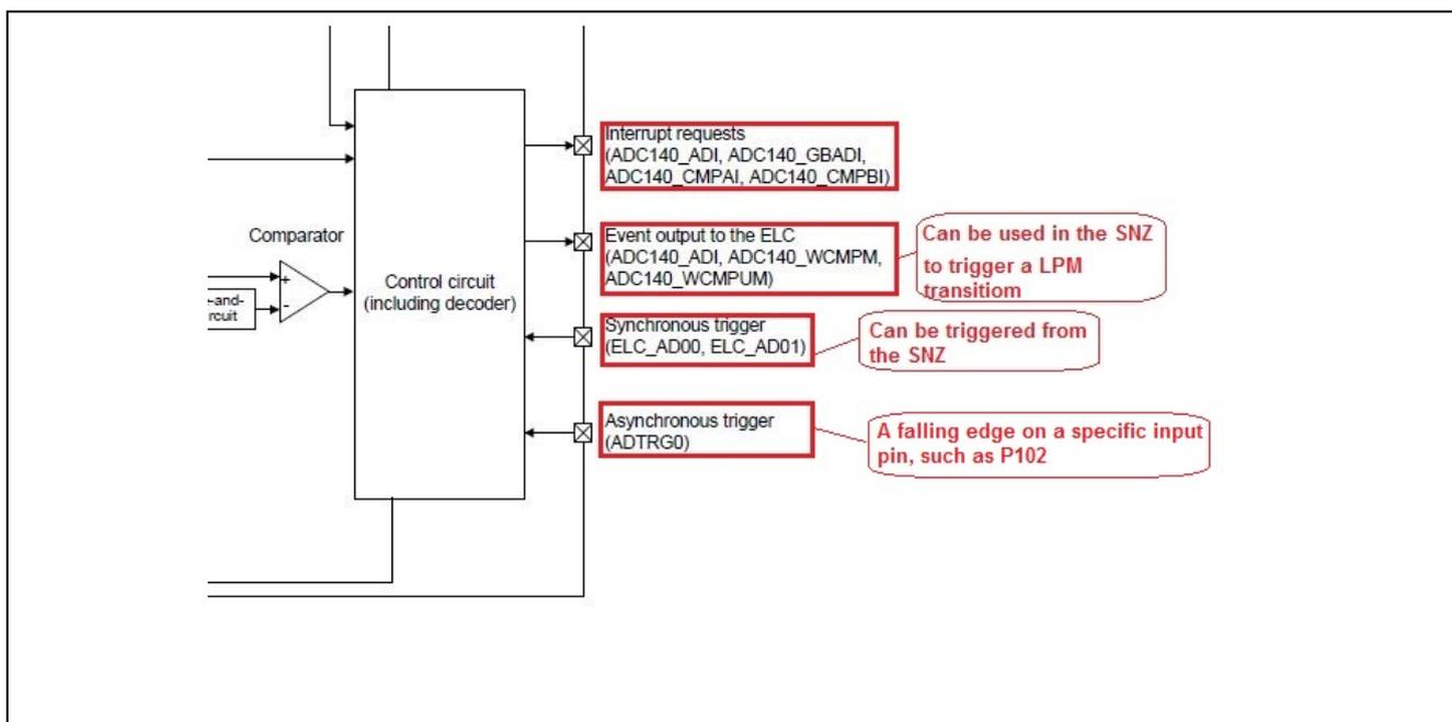
**Figure 8. Input and output events for ADC14**
