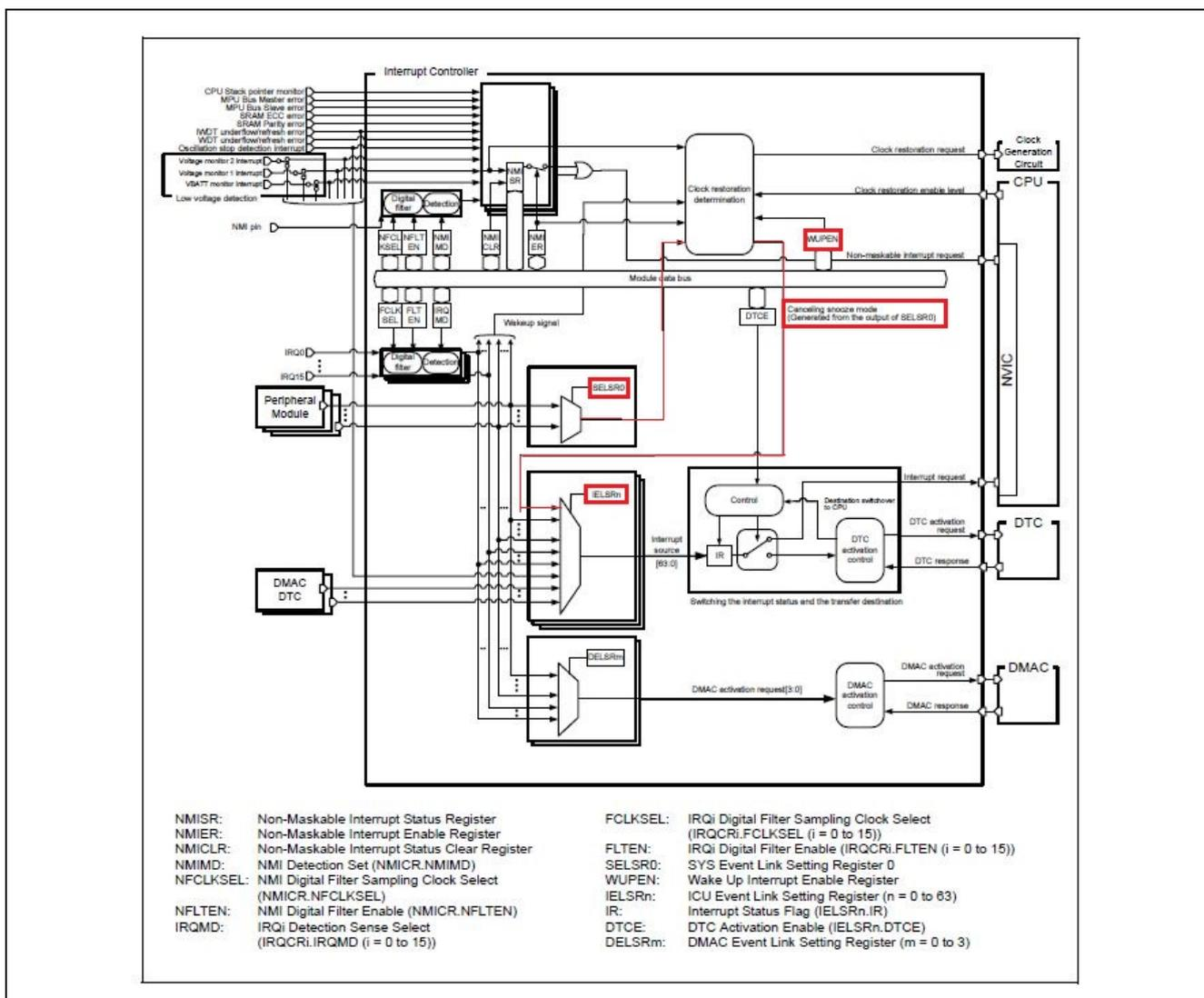
**Figure 6. ICU functional blocks for waking up the LPM**
