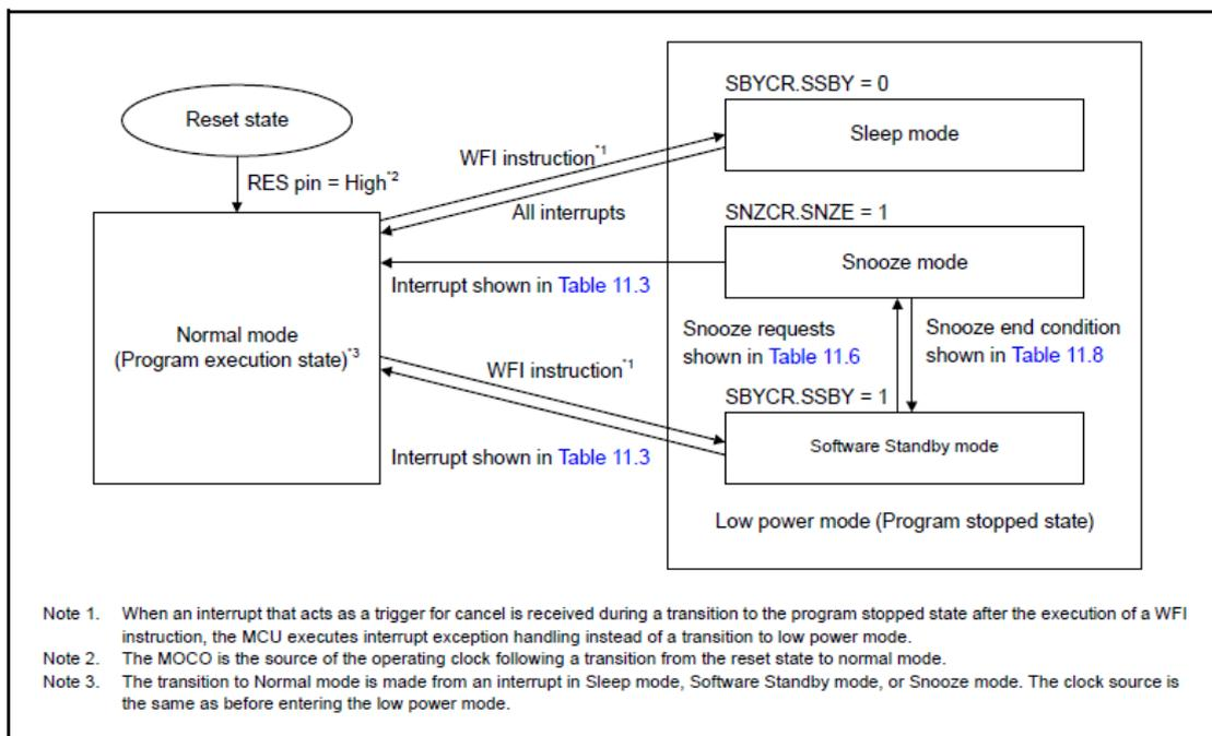
**Figure 4. Possible LPM transitions for S3A7 MCU**
