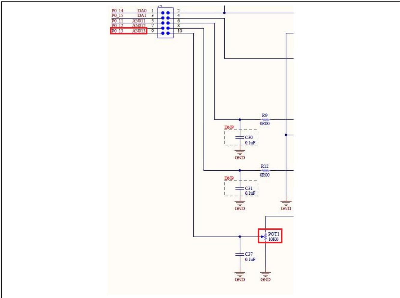
Figure 7. Potentiometer connection to the analog channel 13 on DK-S3A7
