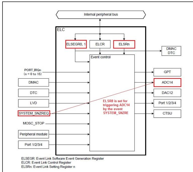
**Figure 5. Selecting a proper source event to trigger a peripheral operation in ELC**
