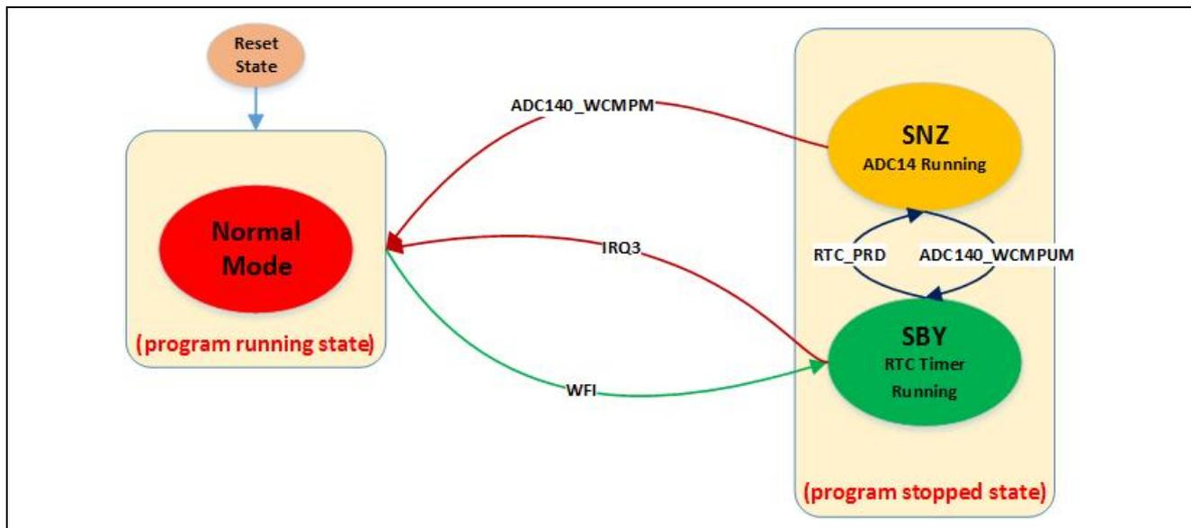
Figure 3. MCU states and LPM transitions used in this application
