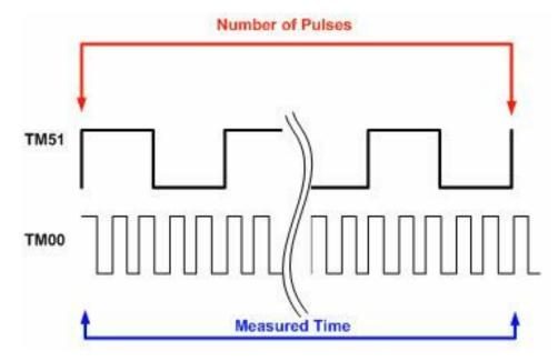
Figure 3-4 Measuring oscillator frequency
