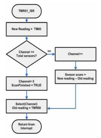
Figure 5-2 Flowchart "Interrupt service routine"
