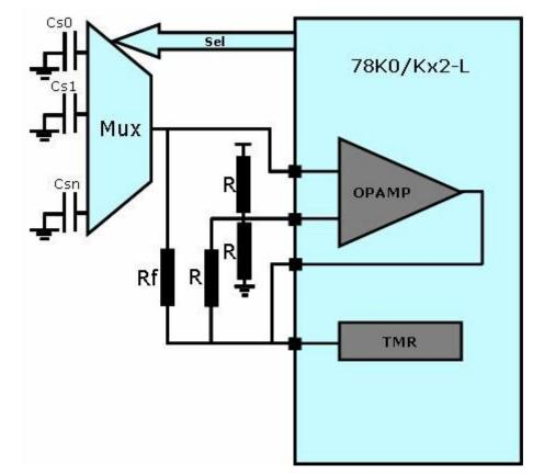
Figure 4-2 Multiple sensor connections
