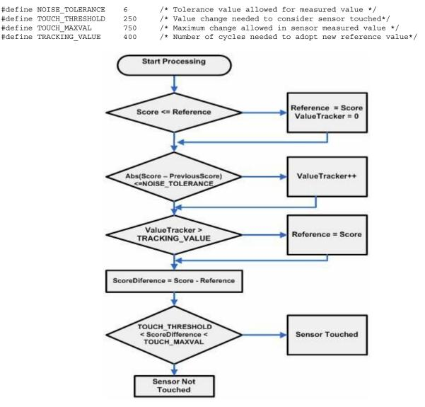
Figure 5-3 Flowchart "Processing measured values"
