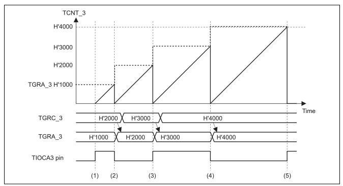
Figure 2 Timing of Pulse Output Operation
