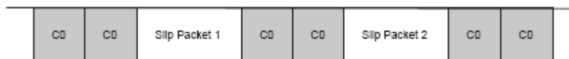
図 4-1 SLIP Packets with 0xC0 at the Start and End of Each Packet
