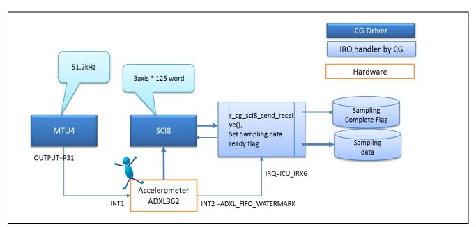
Figure 5-3 Respiratory Rate Measuring Digital Interconnect
