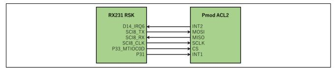
Figure 5-1 Hardware Block Diagram
