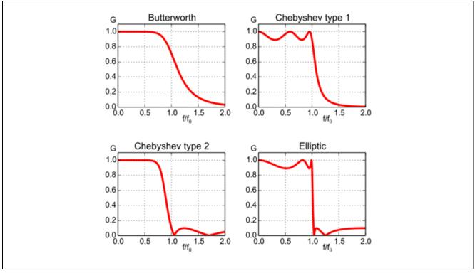
Figure 3-2 Gain distribution of discrete-time filters
