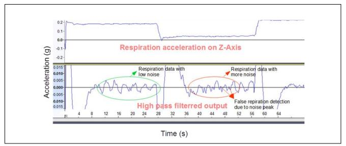
Figure 3-4 False respiration detection due to noise peaks
