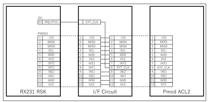
Figure 5-2 Hardware wiring chart
