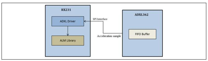
Figure 5-3 Interface of the ADXL362 Sensor with the MCU
