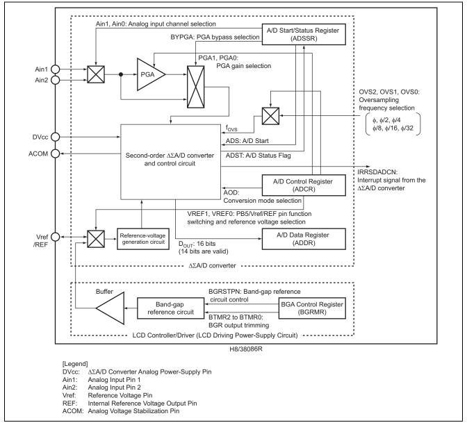
Figure 3 Block Diagram of the  $\Delta\Sigma A/D$  Converter
