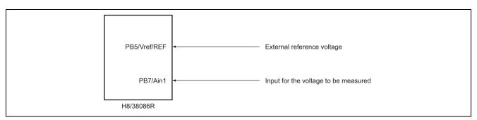
Figure 1 Setup of the  $\Delta\Sigma A/D$  Converter for Measurement Results to be Averaged
