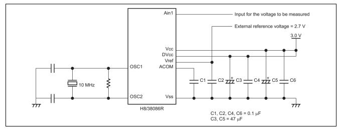
Figure 2 ΔΣΑ/D Converter Measuring Circuit (When Using an External Reference Voltage)
