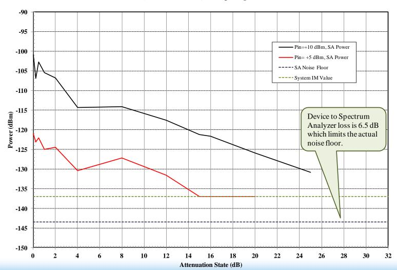
F1950 IM3 Power Levels +25 C, FC = 3.500 GHz, Tone spacing = 60 MHz
