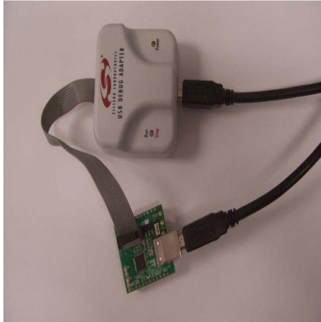
FIGURE 2. SILICON LAB USB DEBUG ADAPTER HOOK UP FOR THE INTERSIL USB DONGLE
