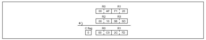
Figure 4.3 Example of Addition with Upper Bits Unused
