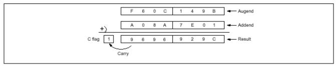
Figure 4.1 Example of Addition with a Carry
