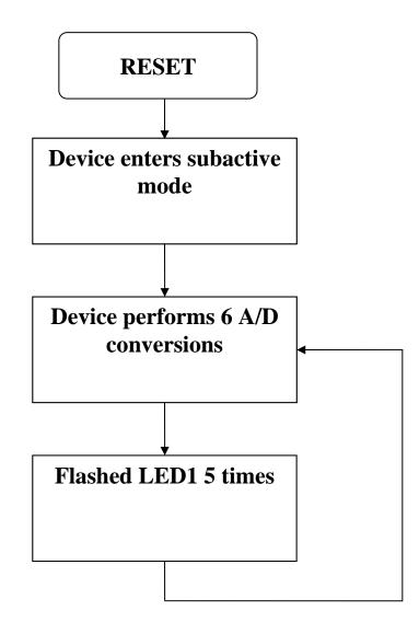
Figure 3: Program Flow for Debug configuration
