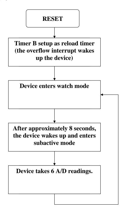
Figure 2: Program flow for Release Build
