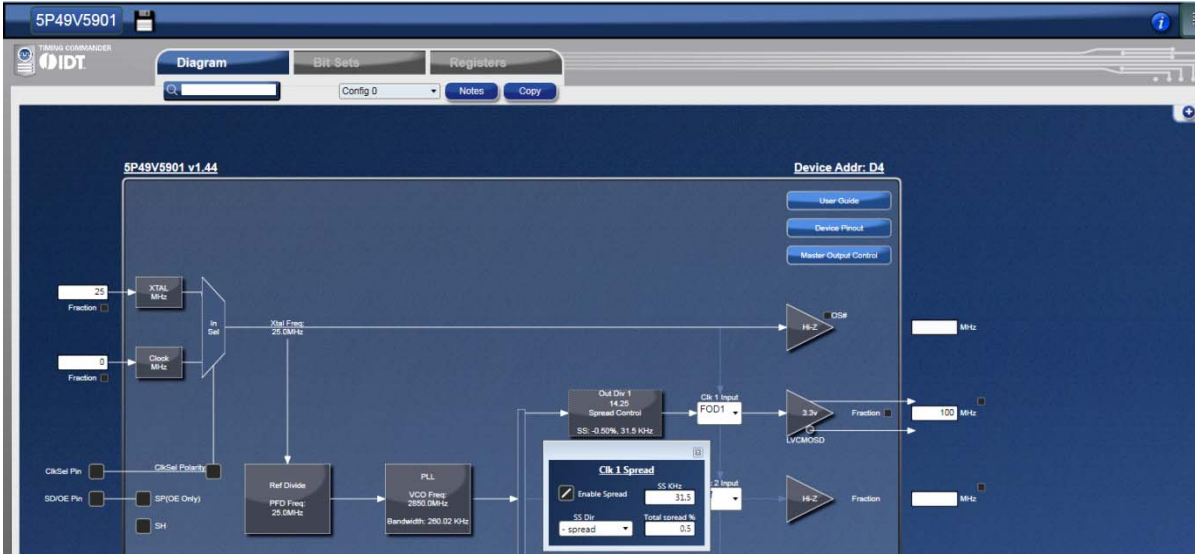
Figure 5. Timing Commander Example of Programming FOD1
