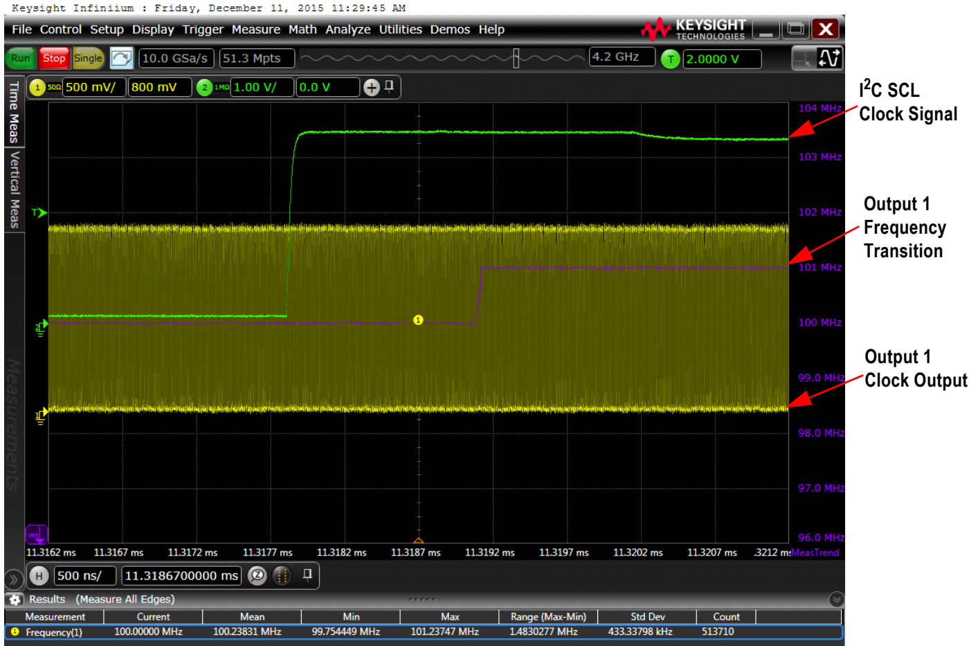
Figure 4. Frequency Transition from 100MHz to 101MHz
