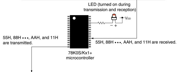
● Transmission test (received 8 units of data are transmitted)
