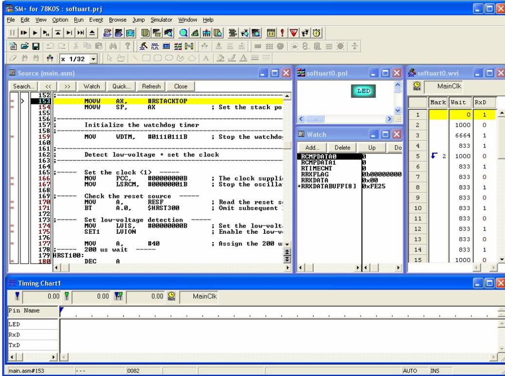
(3) The first character changes from a plus sign (“+”) to a minus sign (“-”) and the receive data to be saved will be expanded and displayed below “-RRXDATA [8]”, by selecting the watch window (Watch) and double-clicking “+RRXDATA [8]”.
