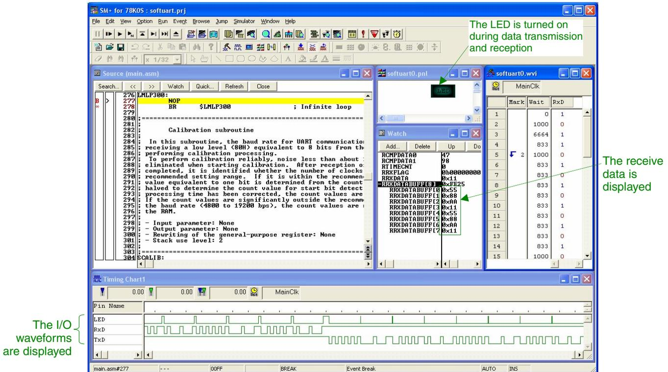
(8) The I/O waveforms will be displayed in the timing chart window and the received data will be displayed in the watch window as follows.
