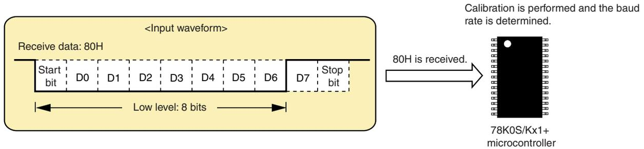
After completion of calibration, 8 units of data are received as a reception test, which are transmitted as a transmission test. Furthermore, an LED is turned on during transmission and reception.
