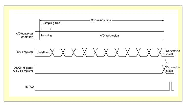
Figure 1-1. Basic A/D Converter Operation (A/D Conversion: 1 Time)
