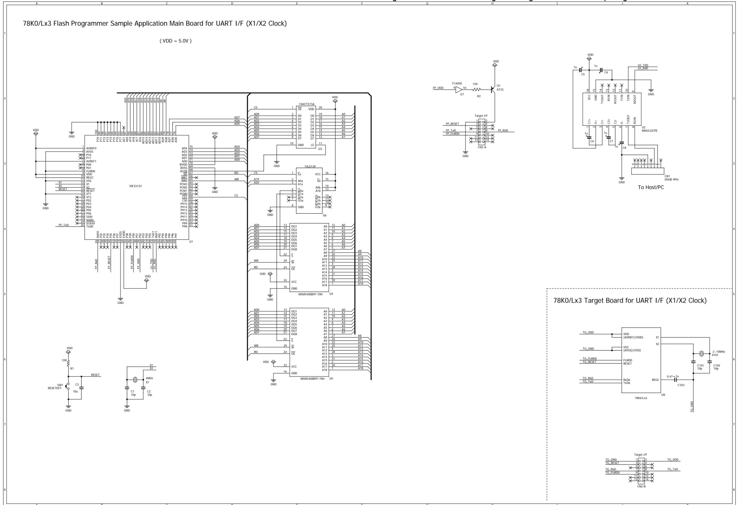
Figure A-2. Reference Circuit Diagram of Programmer and 78K0/Lx3 (During UART communication: with External Clock Used)
