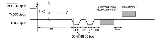
Remark TxD: TxD6 RxD: RxD6 (e) Chip Erase command/Block Erase command/ Block Blank Check command/Oscillating Frequency Set command
