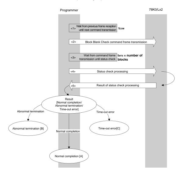
Block Blank Check command processing sequence
