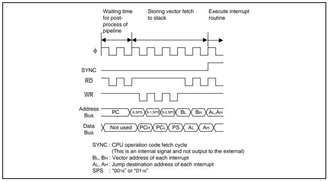
Figure 3.5 Timing Chart of Interrupt Process
