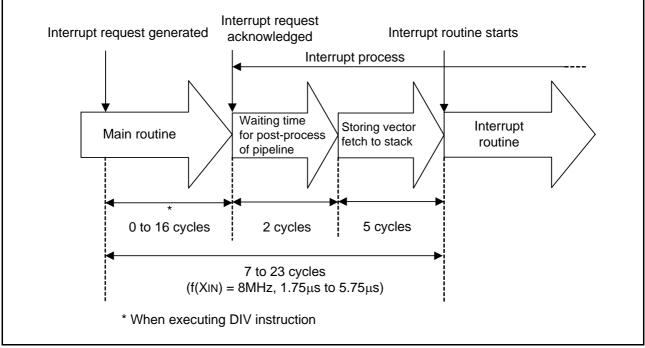
Figure 3.4 Time up to Execution of Interrupt Routine
