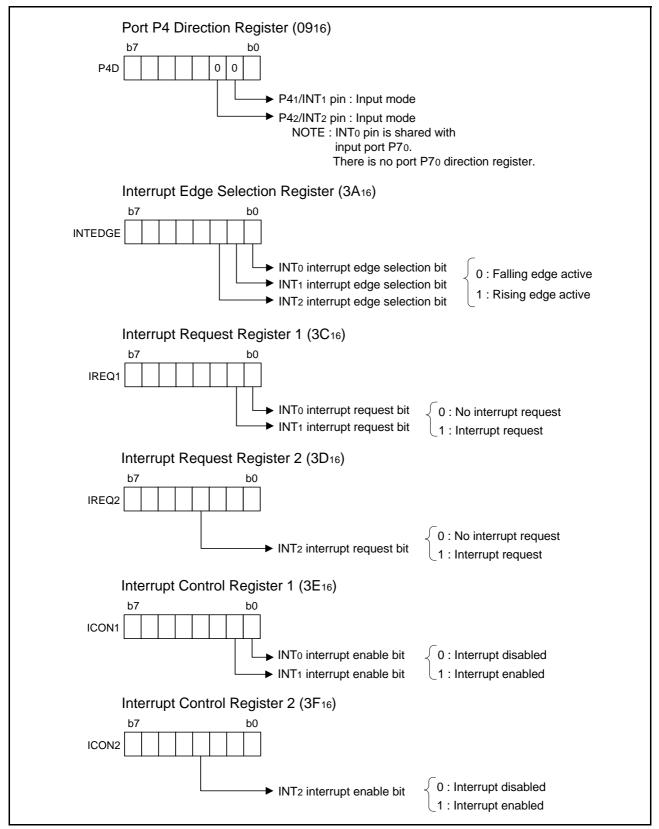
Figure 3.7 Relevant Registers Setting
