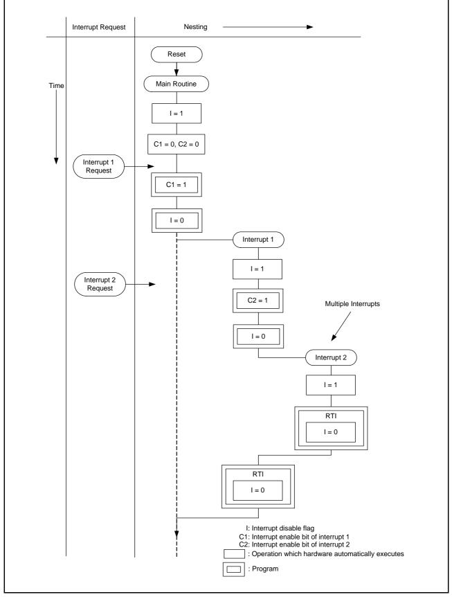
Figure 3.6 Example of Multiple Interrupts
