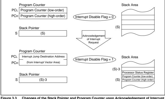
Figure 3.3 Changes of the Stack Pointer and Program Counter upon Acknowledgement of Interrupt Request
