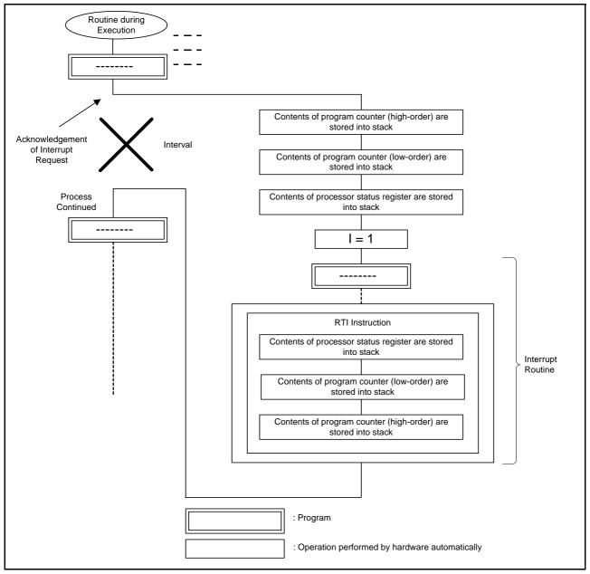
Figure 3.2 Interrupt Operation Diagram
