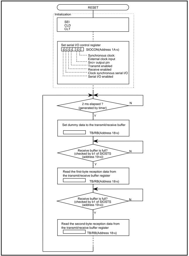
Figure 6 Control procedure of receiver
