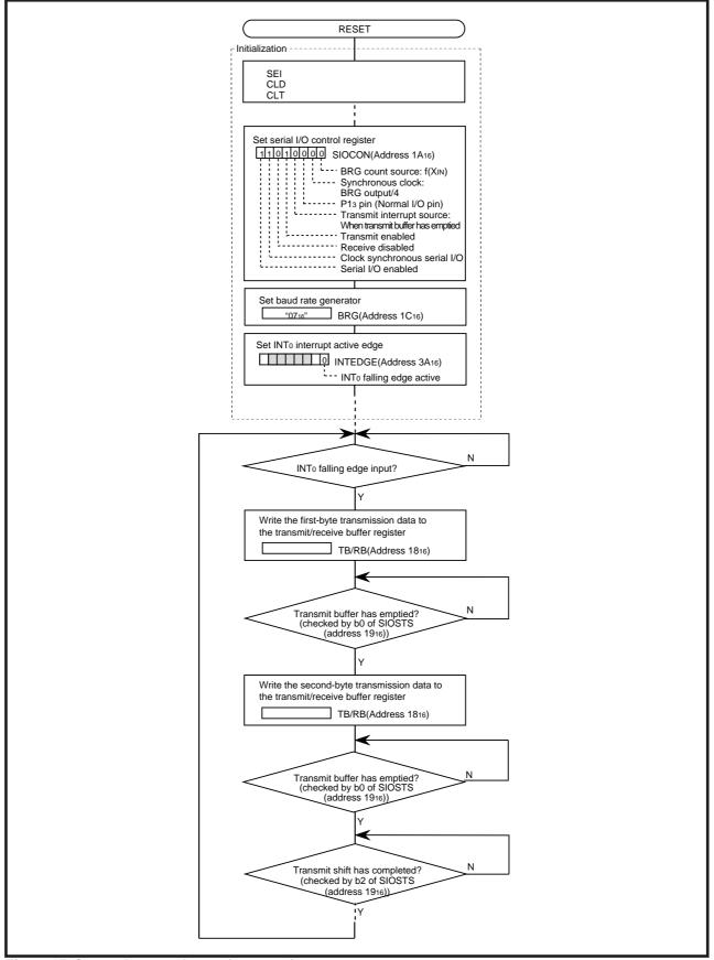
Figure 5 Control procedure of transmitter
