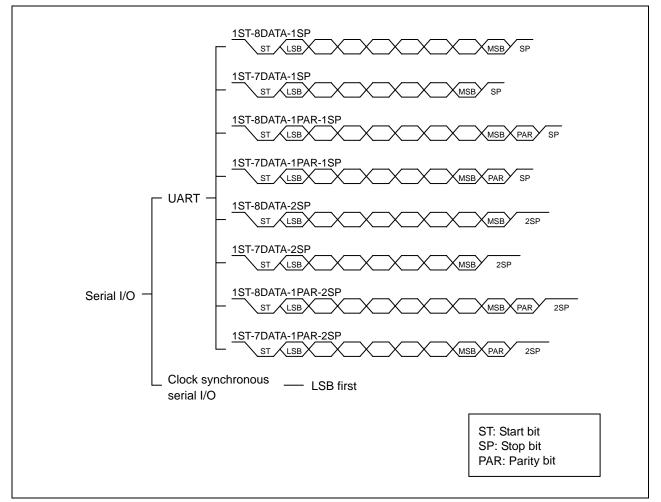
Figure 3.3 Serial I/O Transfer Data Format
