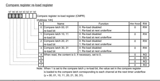
Fig. 4.13 Configuration of Compare register re-load register
