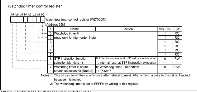
Fig.4.47 Configuration of Watchdog timer control register
