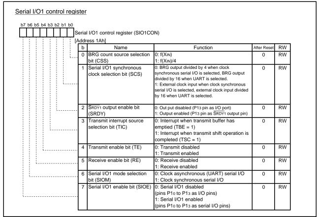
Fig. 4.19 Configuration of Serial I/O1 control register
