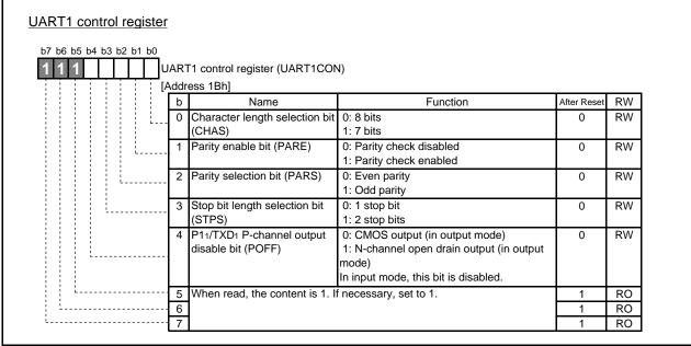
Fig. 4.20 Configuration of UART1 control register
