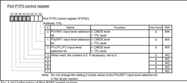
Fig. 4.16 Configuration of Port P1P3 control register
