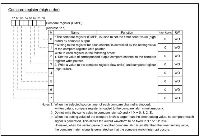
Fig.4.10 Configuration of Compare register (high-order)
