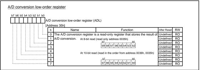
Fig.4.43 Configuration of A/D conversion low-order register
