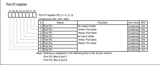
Fig. 4.1 Configuration of Port Pi register (i = 0, 2, 3)
