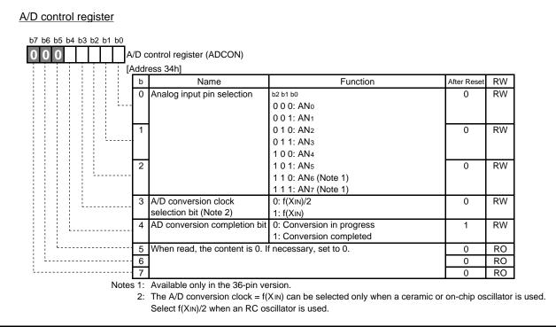
Fig.4.42 Configuration of A/D control register
