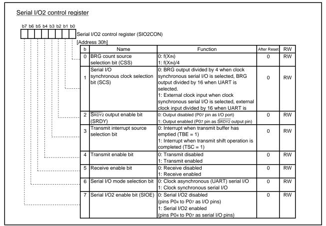
Fig.4.39 Configuration of Serial I/O2 control register
