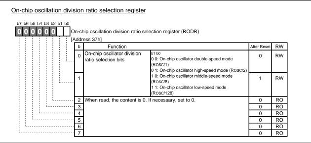
Fig.4.45 Configuration of On-chip oscillation division ratio selection register
