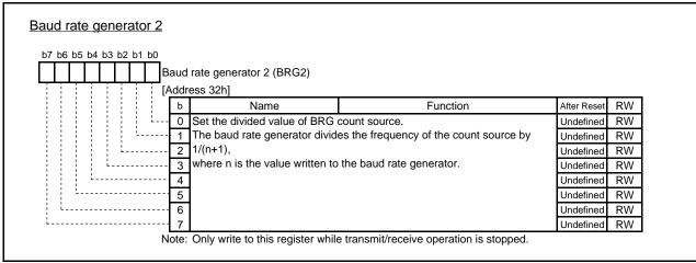
Fig.4.41 Configuration of Baud rate generator 2
