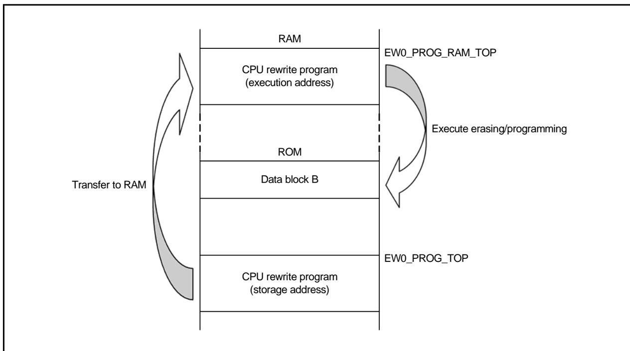
Figure 3.2 CPU Rewrite Program Allocation Map
